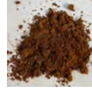
Sample of sand taken from the landscape to the North East of the school building. The location is shown in previous report dated 2020. This is a pure, clean sand with no clay material or lime particles. It has been washed and graded over-time to successive glacial melt-water action. This sand is perfect for use within a clay plaster.
